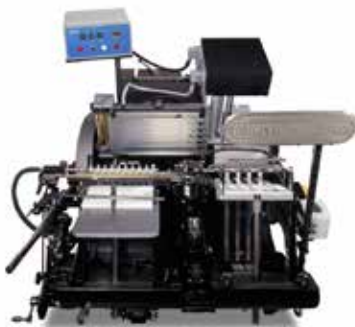
Pro Line Platen Press with Starfoil foil conversion unit
