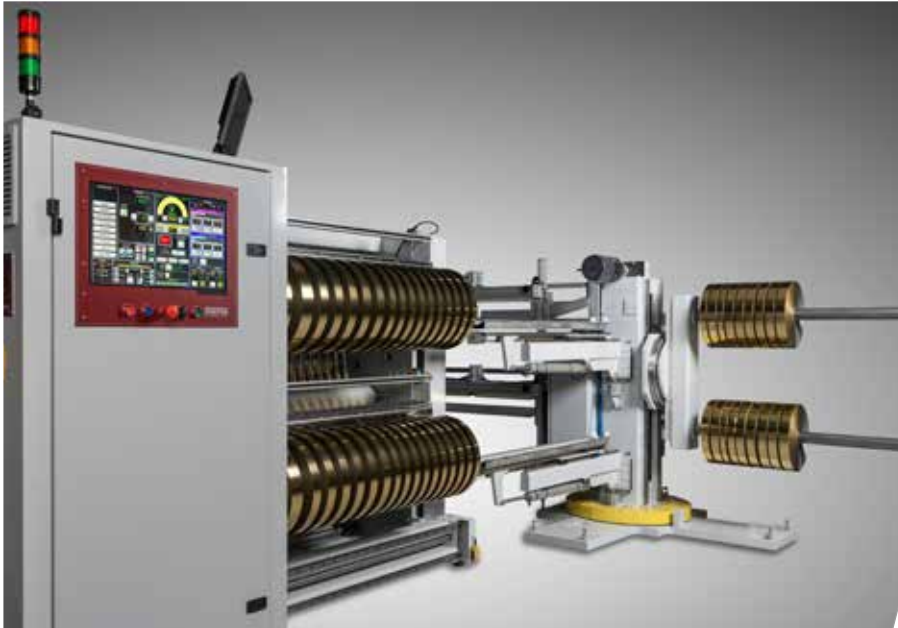
Automatic core loading / Automatic offloading robot
