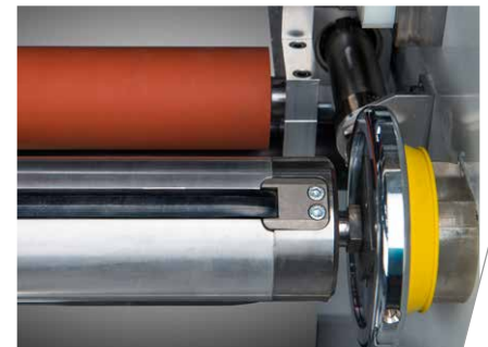
Lay on rollers
